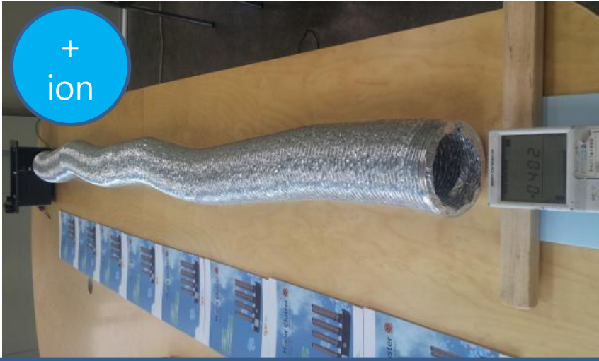
402,000 sets/cm 3 (200cm away with 60mh fan and flexible duct)
