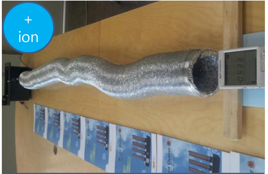
533,000 sets/cm 3 (150cm away with 60cmh fan and flexible duct)
